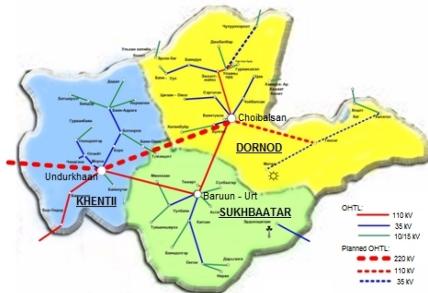
Figure 3-11. ERES Transmission line scheme
